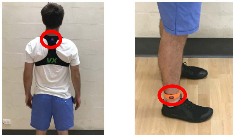
Figure 1. Position of the VX Sport IMU and two Vicon Blue Trident IMUs during movement circuit.
